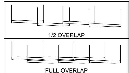
Offers two basic overlap methods. With holes on 1" centers, most any overlap is possible.
